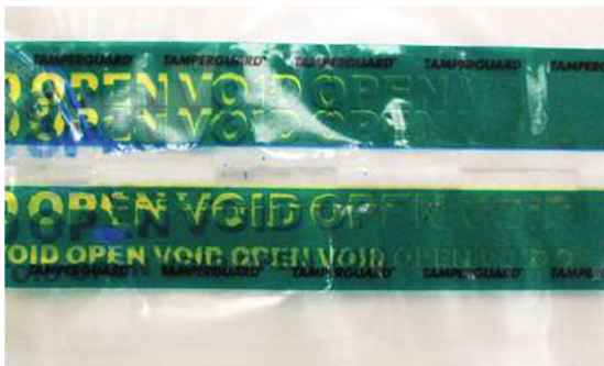
Obvious sign of tampering
